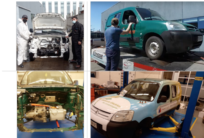
Fig. 11.3: Electric car retrofit process.
