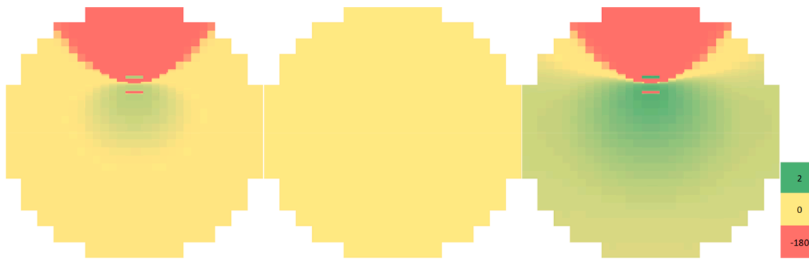
Fig. 26. The phase of thermal neutron noise in the original EOC 39 core loading (at the mid-height position of the detector installation) - Left: Total noise, Center: Point kinetics component, Right: Shape function.
