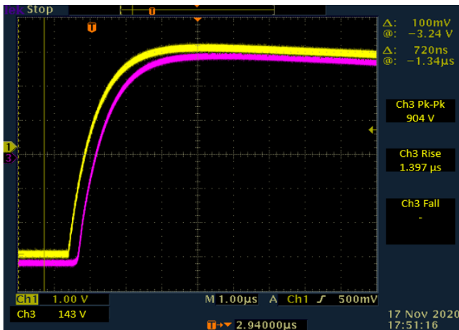
Fig. 4. Example of a 900 V LI superimposed on a - 450 V DC
