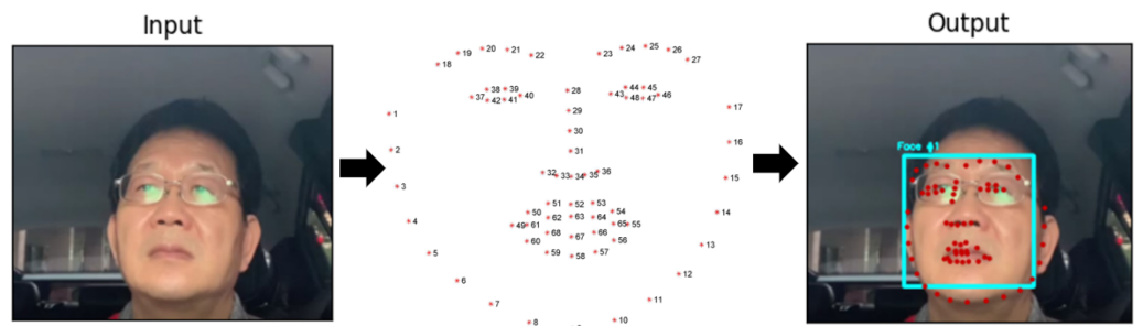
Figure 1 Eye detection process using facial landmarks (right eye points = 36–41, left eye points = 42–47).
