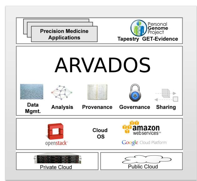
Figure 2: Arvados is a community-driven free software project that extends popular cloud operating systems such as OpenStack or Amazon Web Services. It is designed to run on-premise or hosted. Arvados creates an abstraction between the informatician and the biomedical data management, analysis, provenance, governance and sharing requirements of precision medicine applications. It also enables easy portability across cloud operating systems.
