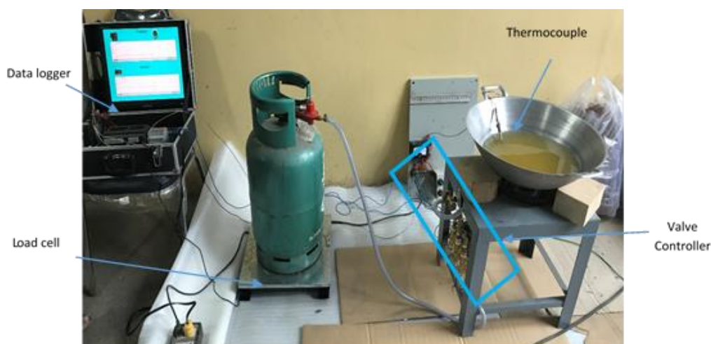
Figure 6. Setup for testing the control system with a gas cooking stove and a frying pan
