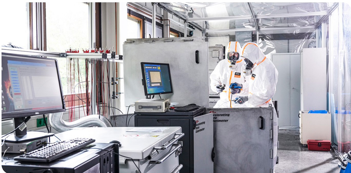
Fig. 4: IAM-AWP Battery Calorimeter Laboratory with seven Accelerating Rate Calorimeters of different sizes
