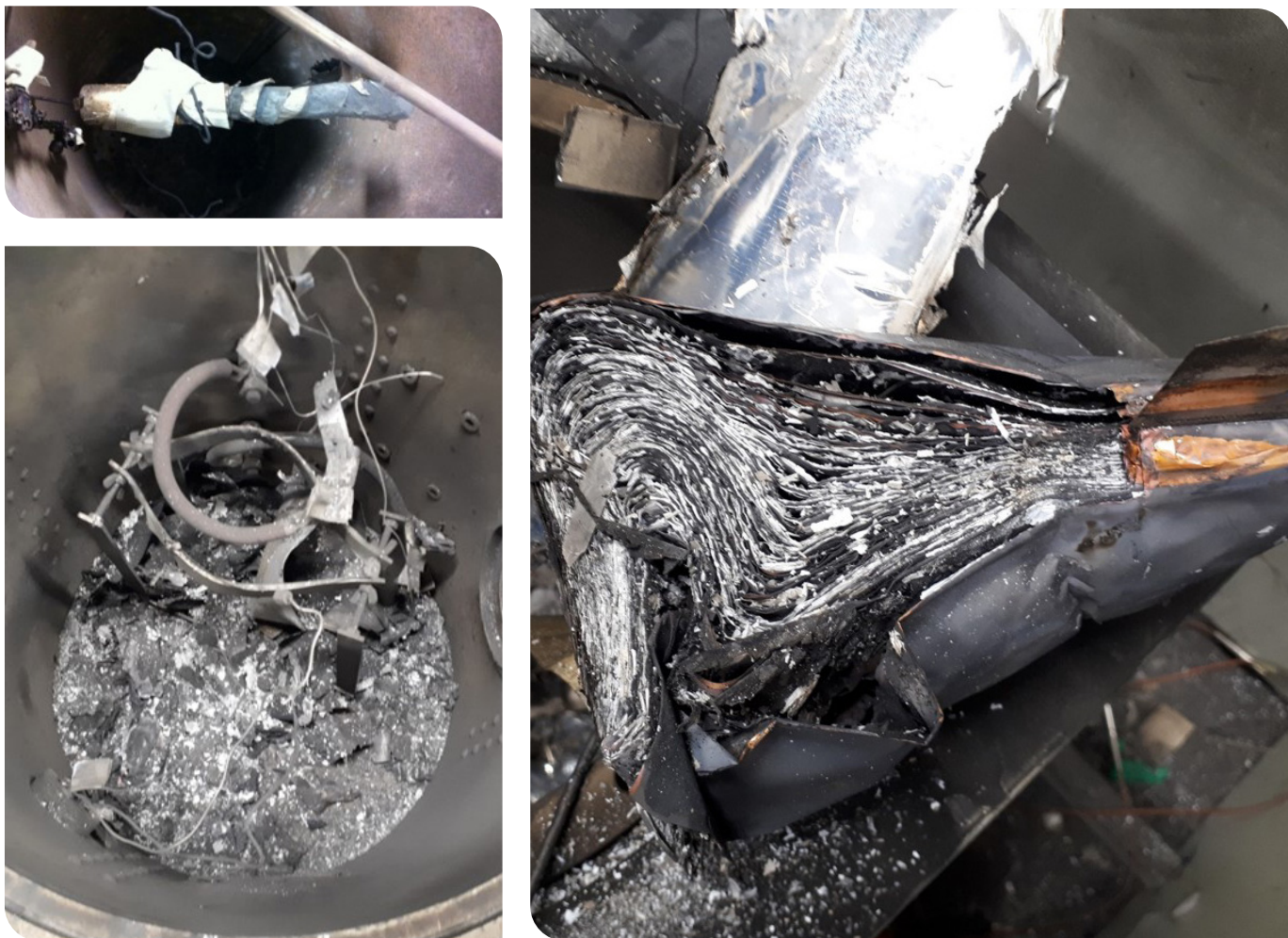
Fig. 6: Examples for cylindrical (top left), prismatic (bottom left) and pouch (right) cells after thermal runaway initiated by an HWS test in an ARC
