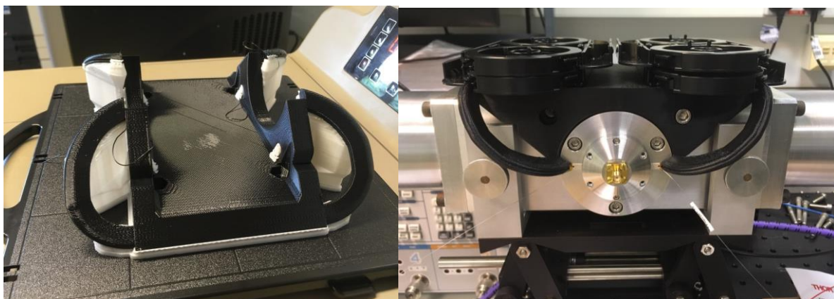
Figure 3 Additive manufacture of the support for the fibre management system and installation on the coaxial line with EO pick-up Grant Agreement 101004730
