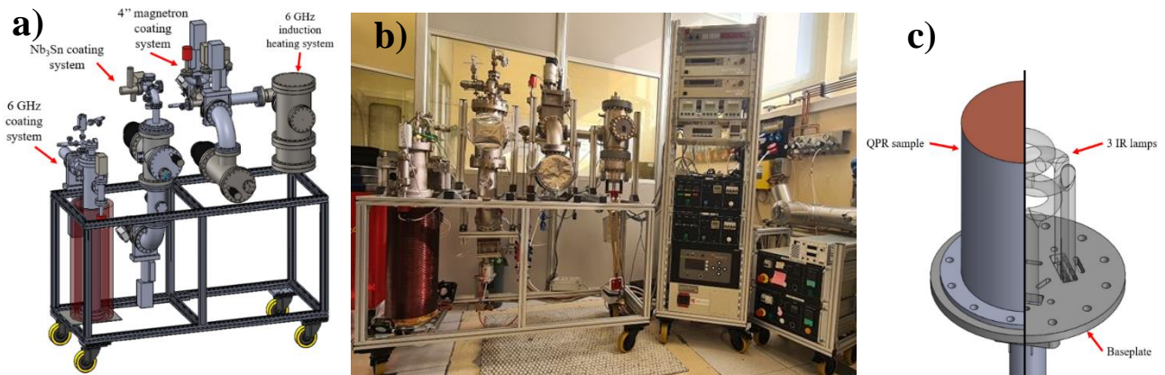
Figure 6: A15 Coating facilities at LNL dedicated to i.FAST project. (a) 3D drawing of the structure containing the 3 coating systems used (6 GHz cavity, Nb 3 Sn QPR, 4" Magnetron coating system used for Nb buffer layer coatings). (b) Picture of the coating facilities installed at LNL. (c) Cross-section of the sample holder used for QPR coating. You can see the 3 lamps that allow substrate temperatures up to 900°C.
