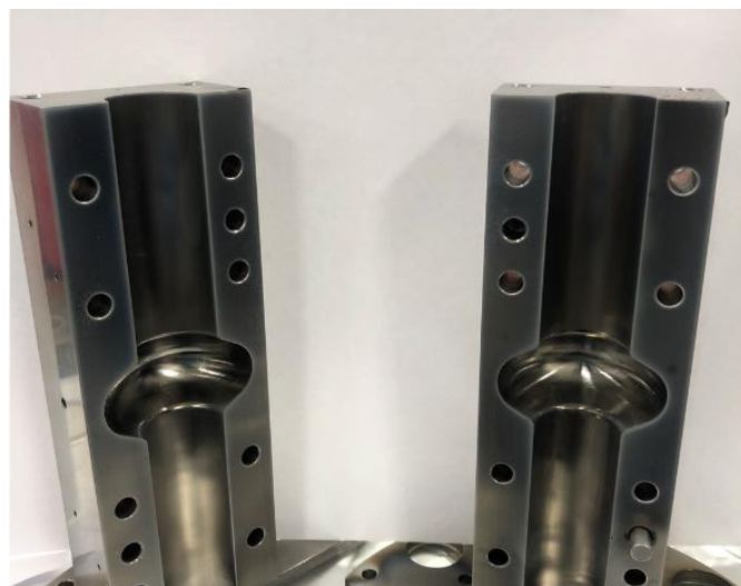
Figure 3: Nb coated open cavity.
