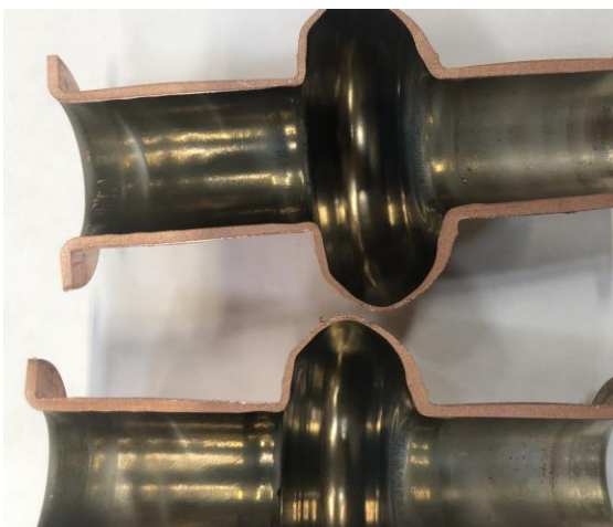
Figure 8: A 6-GHz closed copper cavity deposited with double layer Nb/NbTiN.
