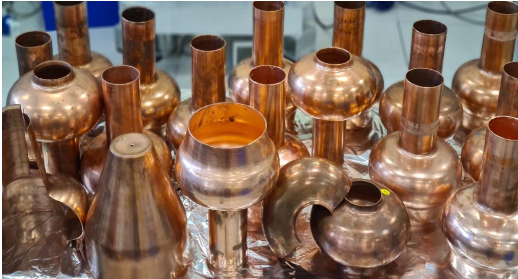
Figure 1: 1.3 GHz seamless copper cavities produced in this work to optimize the CNC program, study the effect of different annealing temperatures and the reproducibility of the process.
