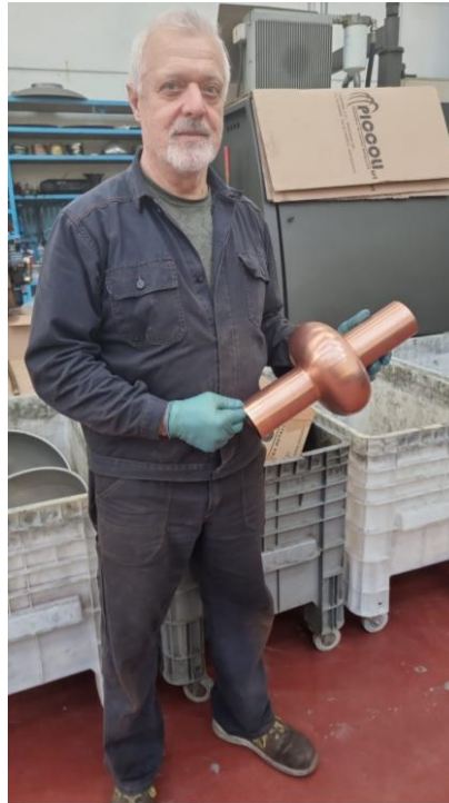
Figure 11: Franco Telatin holding the first complete copper 1.3 GHz seamless cavity made in the iFAST project.
