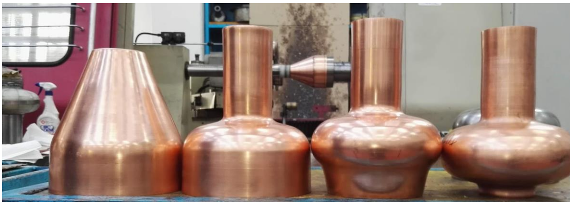
Figure 3: The 4 steps required for the fabrication of elliptical seamless cavities via CNC. In the first two steps (starting from the left), one-piece steel molds are used, while for the following two, Teflon sector molds are used. An intermediate annealing can be done between step 3 and 4 to relax the material and reduce the risk of cracking when closing the second part of the cell.
