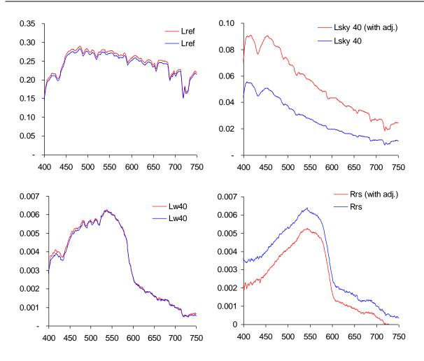
**Figure 1.** Radiances (in  $Wm^{-2}sr^{-1}nm^{-1}$ ) measured in a coastal station in Lake Maggiore (in less than 2 min.) and the related computation of a  $Rrs=(Lw-0.028\cdot Lsky)/(\pi\cdot Lref/pref)$  (where pref is the Spectralon panel reflectance). The Lsky plot clearly shows the increase of the signal due to the contamination of adjacent lands and its impact on the Rrs spectra is not negligible.
