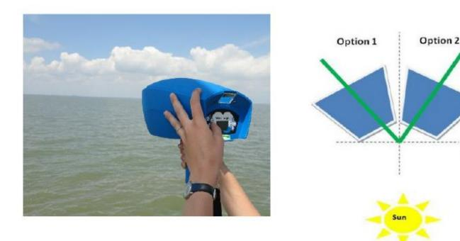
Annex 1, Figure 1. Correct positioning of the WISP-3 during the measurement
