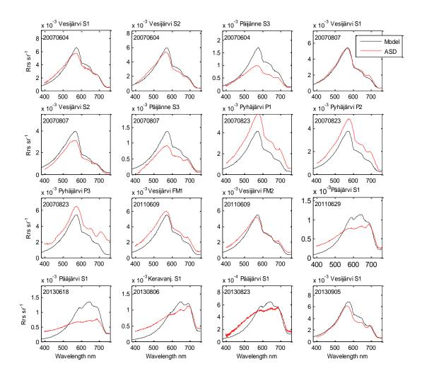
**Figure 3**. Rrs measured with ASD FR instrument and simulated with Hydrolight in Finnish lakes. Measurement dates (yyyymmdd) are also presented. Note different values on y-axis.
