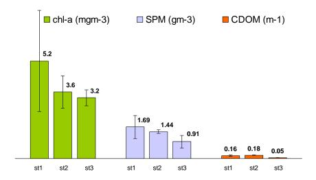
**Figure 10.** Chl a, SPM and CDOM concentrations in three stations measured on 30<sup>th</sup> of September 2014 in Lake Garda. Each bar shows the average value (with standard deviation) computed from three replicates (for each parameter and site).
