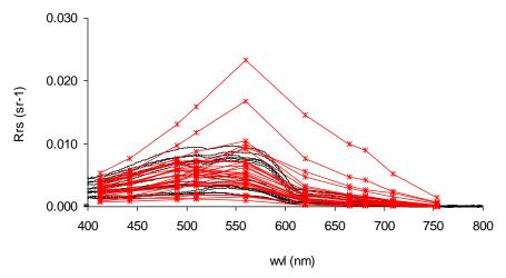
**Figure 5.** Comparison between Hydrolight-simulated (in red for the S3 band setting) and in situ measured (continuous lines in black) Rrs spectra (ASD and WISP-3 data). With respect to Fig. 1, 11 spectra with a suspect degree of bottom-effect contamination were removed.
