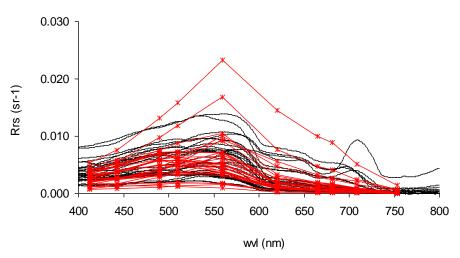
**Figure 4.** Comparison between Hydrolight-simulated (in red for the S3 band setting) and in situ measured (continuous lines in black) Rrs spectra (ASD and WISP-3 data).
