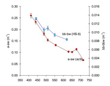
**Figure 12.** In situ absorption and backscattering spectra (all except pure water) acquired on 10<sup>th</sup> of June 2014. The plot shows average values with standard deviations for data acquired at 8 m depth for 10 minutes.
