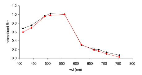
**Figure 6.** Comparison between Hydrolight-simulated (red) and in situ measured (black) Rrs spectra. Each spectrum is the average values of 19 Rrs spectra normalized at 560 nm. The corresponding average values of water quality parameters are Secchi disk 6.08 m, chl-a 1.12 mgm<sup>-3</sup>, TSM 0.94 gm<sup>-3</sup> and CDOM 0.09 m<sup>-1</sup>.
