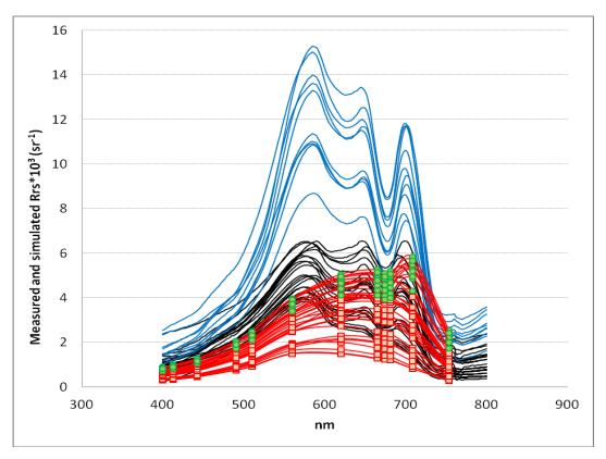
**Figure 8**. Measured Rrs from L. Võrtsjärv (blue line) and L. Peipsi (black line) together with simulated Rrs (red line): S3 channels are represented with green dots (L. Võrtsjärv) and red squares (L. Peipsi).
