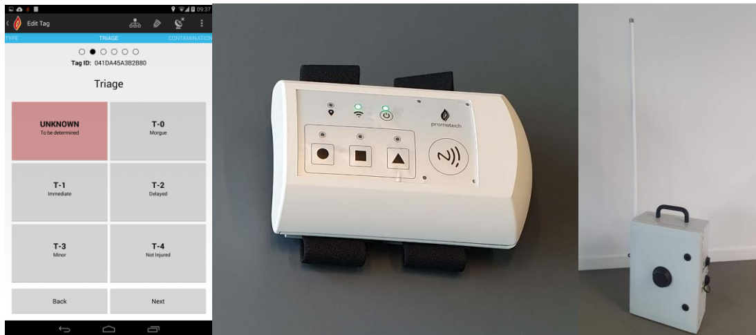
Figure 10: Triage Platform field devices (app, ruggedised tagger and base station)
