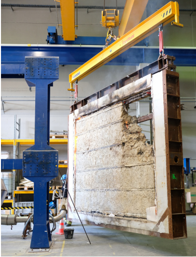
Fig. 22 - Fire resistance test.
