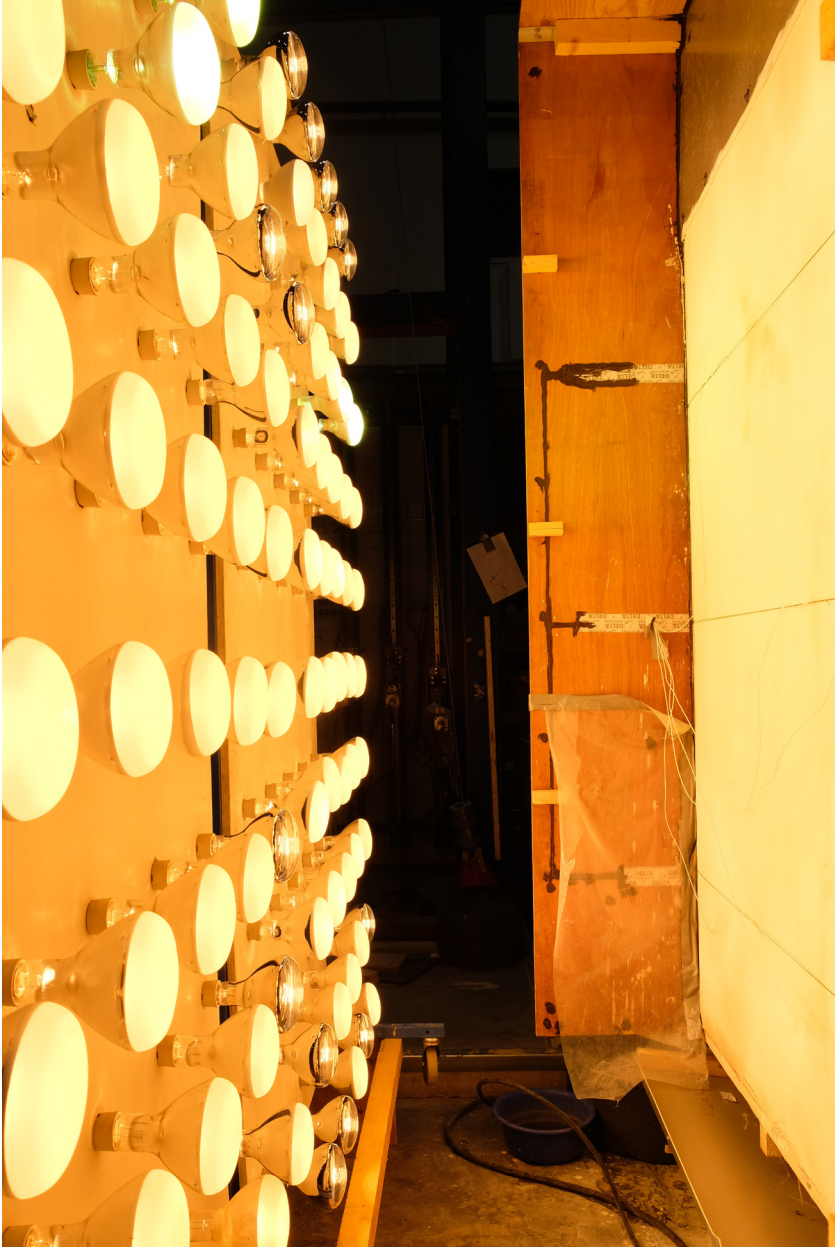
Fig. 24 - The photo shows the drying bench which generates a temperature of 80°C for the drying cycle.
