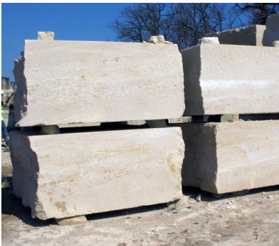
Fig 3 - The blocks extracted from the quarry are waiting to be squared, and to become architectural elements ready to be laid.
