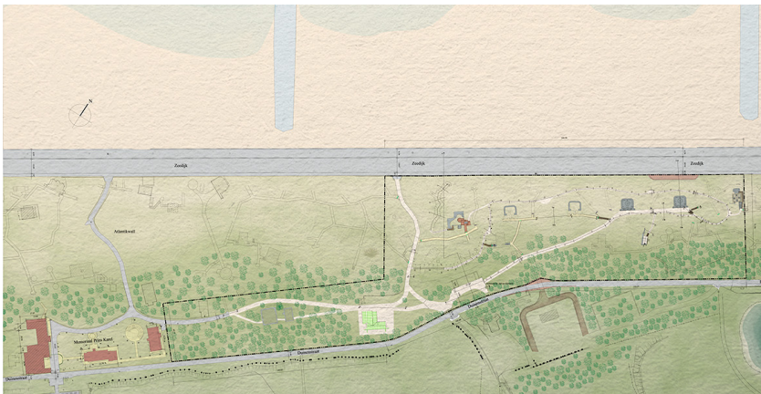
Image 7: project plan for “Batterij Aachen” depicting sea, beach, dunes, routing and artefacts. Project zone indicated by black line, an landscape area of roughly 80.000m2. Credit: aNNo..
