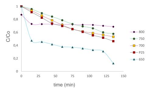
Figure 5. Photocatalytic activity of TiO 2/WO 3 fibers in the photodegradation of methyl orange dye. Source. Authors of the work.
