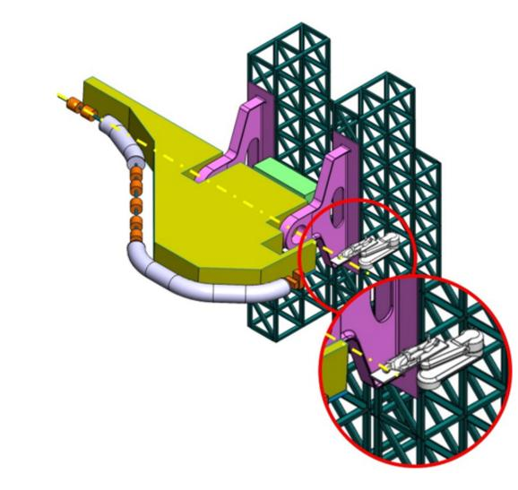
Full Turn Gantry Balanced structure with ground supports; motor drives off-axis friction rollers. Treatment angle range:  $\pm 180^{\circ}$ ; total rotating mass: 120 t.
