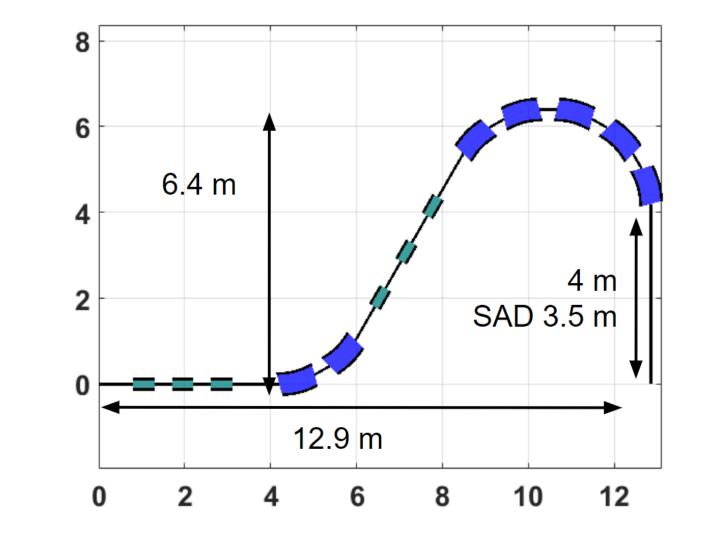
Layout 2 It allows working with a beam momentum spread of 0.1%, in the scenario for which the MF is varied for the same  $\beta$  functions; SC dipoles of 45°.
