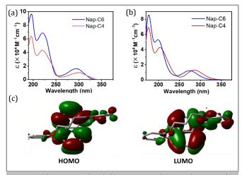
Figure 2 (a) Experimental and (b) computational (TD-DFT/CAM-B3LYP/6-31G(d) level) UV-Vis absorption spectra of Nap-C4 (red) and Nap-C6 (blue). Measured in acetonitrile. (c) Calculated HOMO and LUMO orbitals for Nap-C4.
