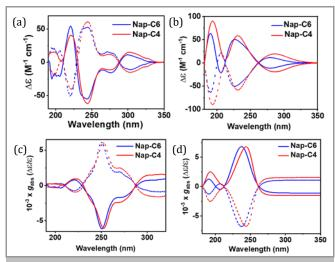
Figure 3 (a) Experimental and (b) computational (TD-DFT/CAM-B3LYP/6-31G(d) level) ECD spectra of Nap-C4 (red) and Nap-C6 (blue). (c) Experimental and (d) computational anisotropy factor. Solid: *P* enantiomers, dashed: *M* enantiomers. Measured in acetonitrile at room temperature.
