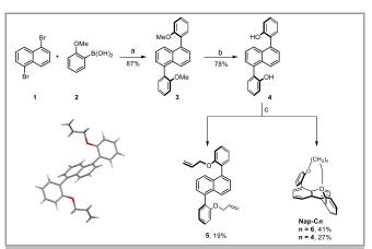
Scheme 1 Synthetic pathway to Nap-Cn. Conditions: (a)  $Pd(PPh_3)_4$ ,  $Na_2CO_3$ , dioxane/water; (b) BBr<sub>3</sub>, dichloromethane,  $0^{\circ}C \rightarrow RT$ ; (c)  $BrCH_2(CH_2)_{n-2}CH_2Br$  (n=3,4,6), KOH, DMSO (*i.e.*, dimethyl sulfoxide). Bottom left: X-ray structure of **5**.
