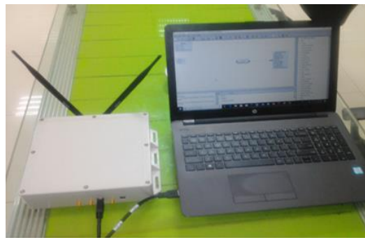
Figure 3. Interconnection of USRP B200 with host PC for real data acquisition campaign
