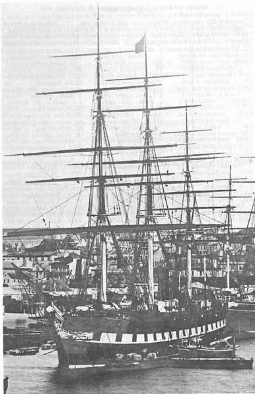
The famous auxiliary ship Great Britain , of 3343 tons, at Circular Quay, Sydney, 1866. She was the first iron screw steamship in the world and was designed to carry over 600 passengers. On the England-Australia run from 1862 to 1876, she probably brought more settlers to Australia than any other ship. Photo from the author's collection. (See further illustration on page 214).
