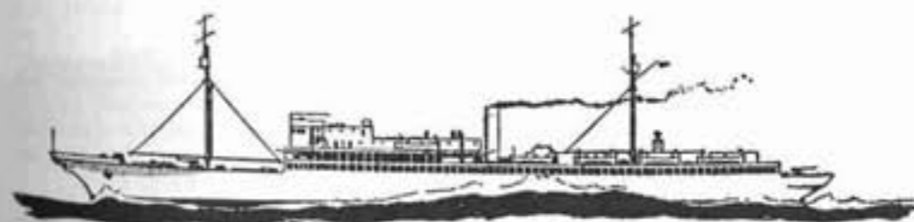
USS Holland , American submarine tender of 8100 tons, built in 1926 & mounted eight 5-inch guns. Based in Australia in 1942-3.
