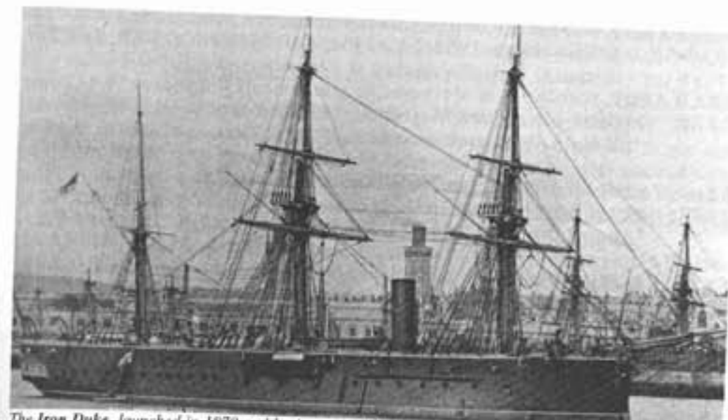
The Iron Duke , launched in 1870 and broken up in 1906, was one of the 'Audacious' class of armoured second-line battleships with an armament of ten 9-inch & four 6-inch muzzle-loading rifled guns.
