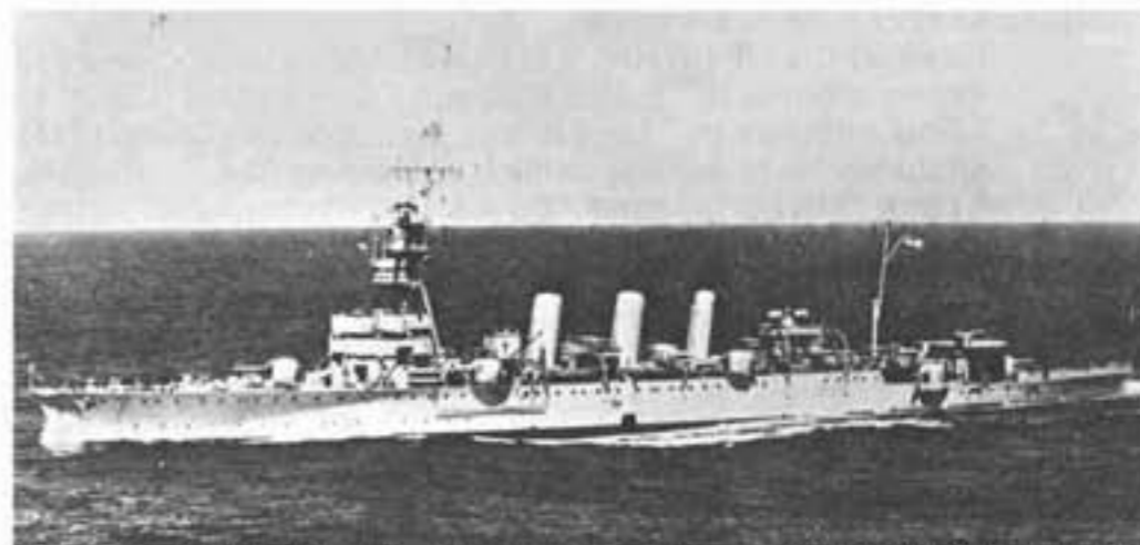
Light cruiser HMAS Adelaide, built at Cockatoo Dockyard Sydney, and completed in 1922, carried nine 6-inch guns and two 21-inch torpedo tubes. She was the oldest British designed cruiser to serve in World War II, & paid off in 1946.
