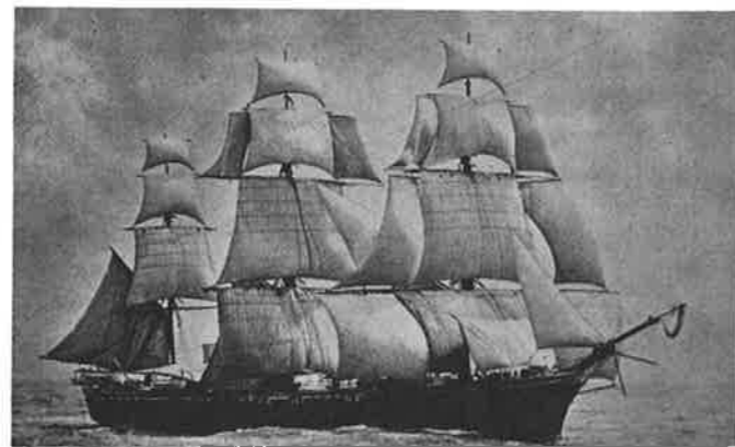
HMS Volage, screw corvette, in the RN Training Squadron c. 1870-1900. Under full sail her funnel is not visible and is probably housed (folded down).
