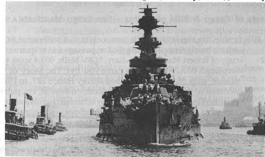
The battleship Malaya leaves New York in pre-war days flanked by a flotilla of tugs. Note the two sailors on the platform on her starboard side - to "heave the lead" and provide depth soundings in the time-honoured method of many centuries.
