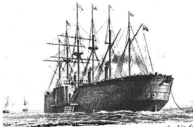
The paddle steamer Great Eastern of almost 20,000 tons was a mammoth ship for her day and well ahead of her times - capable of carrying 3000 passengers. Designed for service to India and the East, she was used on the Atlantic run instead, unsuccessfully, but then made her name laying the trans-Atlantic cable and others. Here her paddle wheels were an advantage as the cable could easily have been caught up in the propellers of a screw steamer, although she was also fitted with a single propeller.
