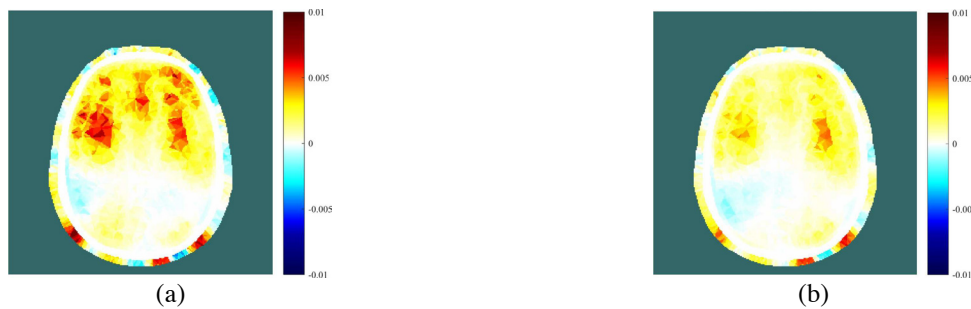
Figure 5. Reconstructed images of REG showing brain perfusion due to the cardiac process : (a) at 300 ms and (b) at 500 ms after the beginning of a ~1-second period cardiac cycle. The measurements were made with fEITER Mk. II.
