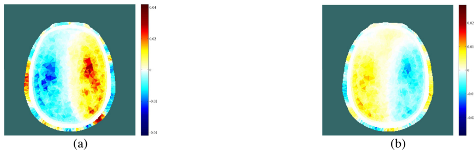
Figure 6. Reconstructed images during (a) left occlusion and (b) right occlusion of THR trials. The measurements were made with fEITER Mk. I.
