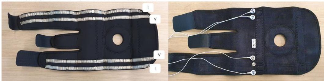
Figure 2. Custom-made brace. LEFT: inside of the brace. (I) shows the outer silver-plated nylon electrodes used for current injecting. (V) are the inner voltage sensing electrodes. Nylon is 1 cm in width. RIGHT: outside of the brace with push buttons to connect the MF BIA device.
