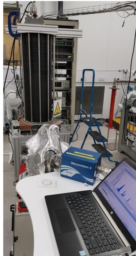
Figure 6: The 1-m NEG deposition vacuum vessel and the magnetic coil prepared for depositing NEG film.
