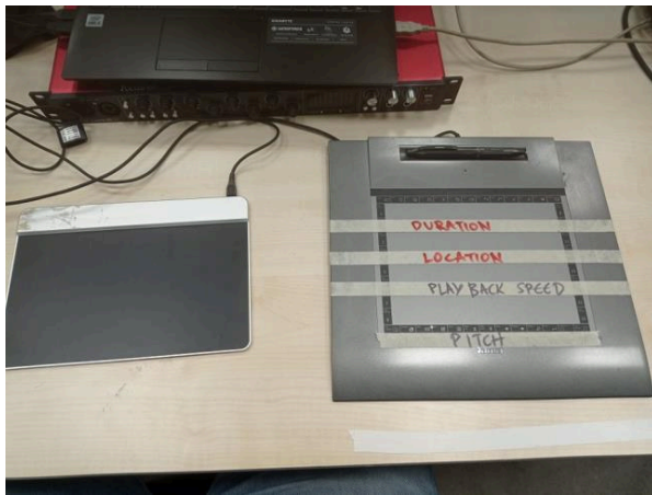
Figure 1. The UI. On the left, the Sensel Morph is located, and on the right is the trackpad for controlling the parameters of the GS synthesis.
