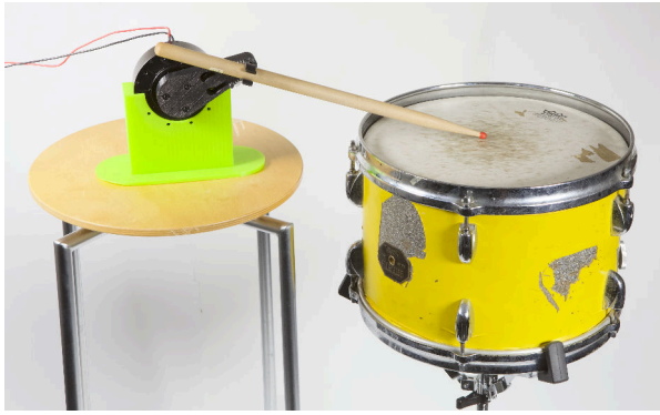
Figure 2: The drum robot playing a snare drum.
