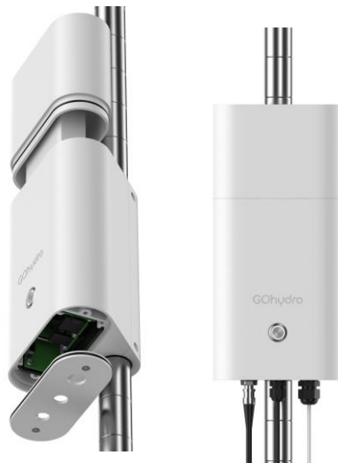
Figure 2.1. Visualizations of the matured All-in-one Sensor Kit concept ready for 3D printing.
