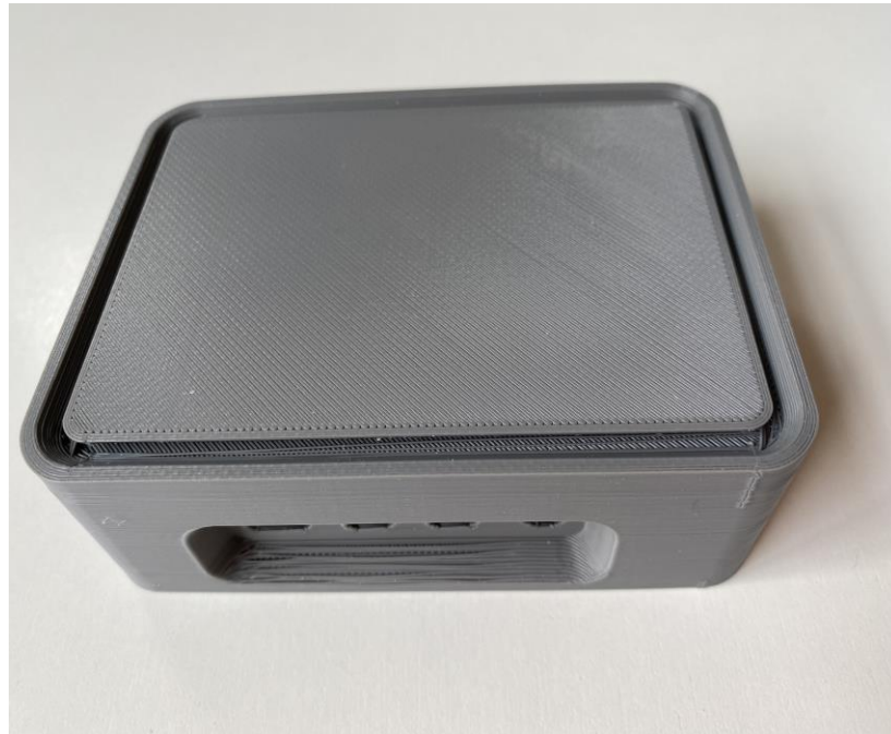
Figure 2.5 3d-printed version of the CSU casing
