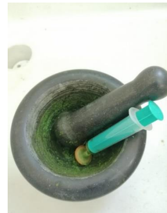
Figure 2.8. Mashing the basil leaves in acetone with a simple pestle and mortar. A syringe with a filter attached to it was used to dispense the liquid into Eppendorf tubes.
