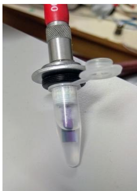
Figure 1.2. Photograph of the photonic chip immersed directly in 2 \mu l of a liquid sample demonstrating the dip-'n'-read measuring format
