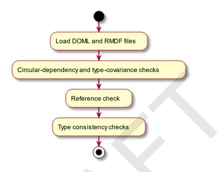
Figure 4. DOML parsing and standard correctness-checking activity diagram.
