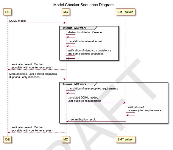
Figure 3. Sequence diagram of the DOML model checker.
