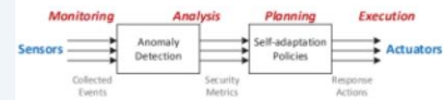
Fig. 2. Anomaly Detection to support monitoring and analysis in the MAPE-K adaptation model.
