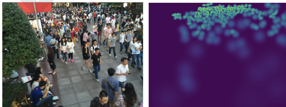
Figure 7: An example image (from the Shanghai Tech crowd counting dataset) and its corresponding ground truth density map.
