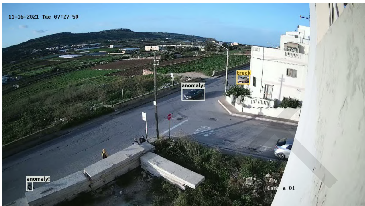
Figure 19: Example frame from the rules based anomaly detector.
