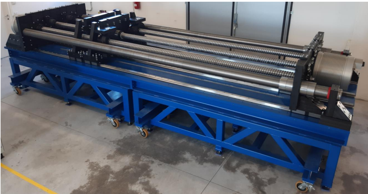
Fig. 14. HIL test rig mechanical assembly.
