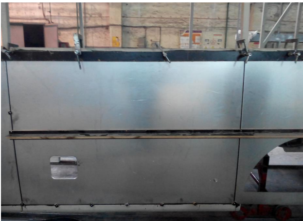
Fig. 9. The body of the bus with glued side panels with double-sided zinc coating
