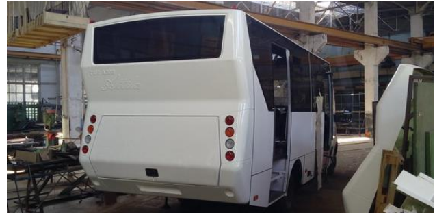
Fig. 10. The body of the bus, the side panels of which are sheathed with polymer sheets with a double-sided coating of aluminum film (the type of Alucobond)
