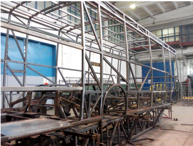
Fig. 2. Bus body frame after welding
