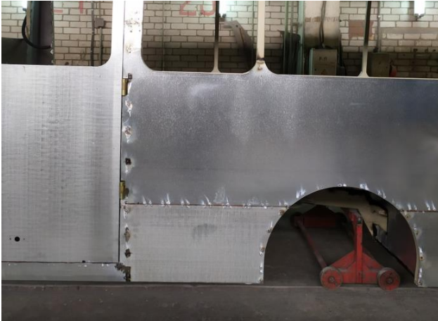
Fig. 5. The body frame of the bus, which has welded cladding with double-sided galvanizing
