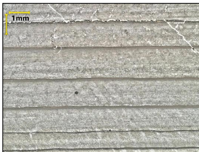
Figure 4: Microscopic investigation of LC-S1 reveals alternating pale and dark layers and upward fining.
