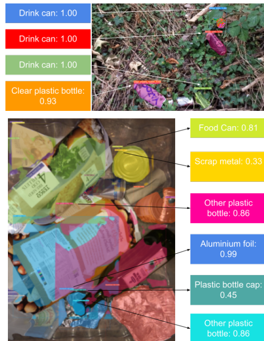
Fig. 7: GarbageNet classification and segmentation: images with single items are classified correctly with high confidence scores (top). Images containing multiple items are classified with smaller confidence score due to occlusions (bottom).
