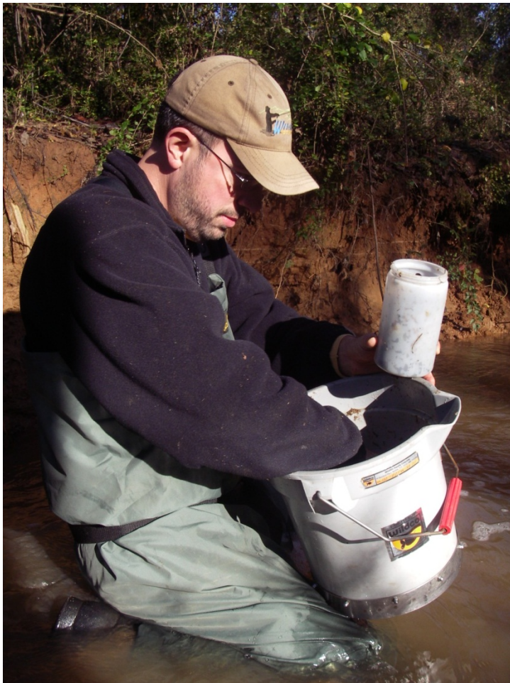
Figure 4-3. Removing a benthic macroinvertebrate sample from a sieve bucket and placing the sample material in a 1-liter container with approximately 95% ethanol preservative
