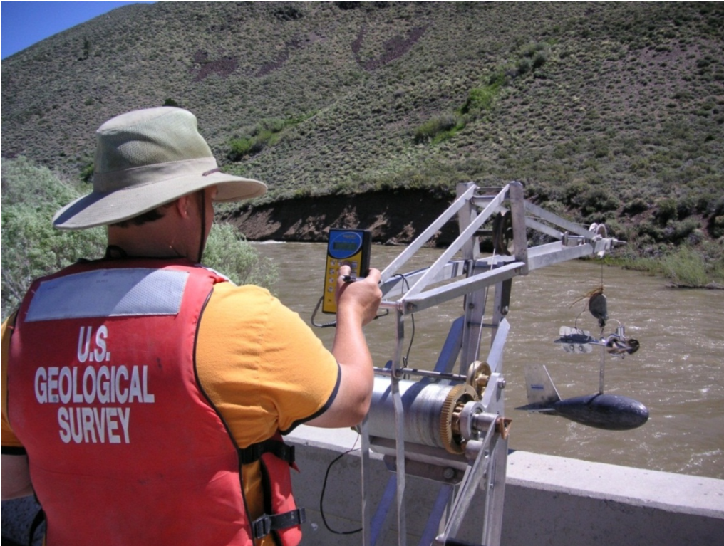
Figure 3-11. Measuring discharge from a bridge using a current meter and crane (USGS n.d.)
