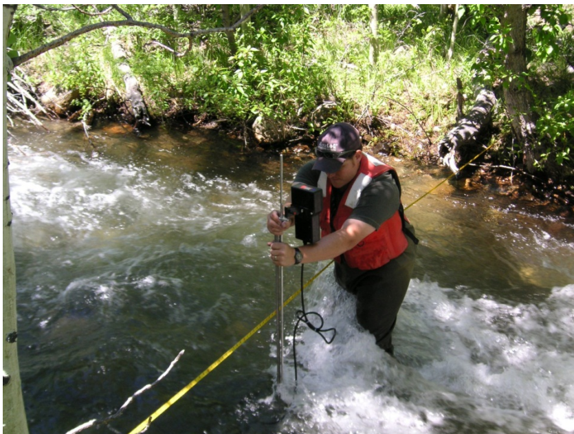
Figure 3-7. Measuring stream discharge (USGS)
