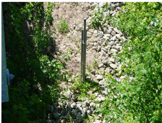
Figure 3-2. Traditional crest-stage gage
