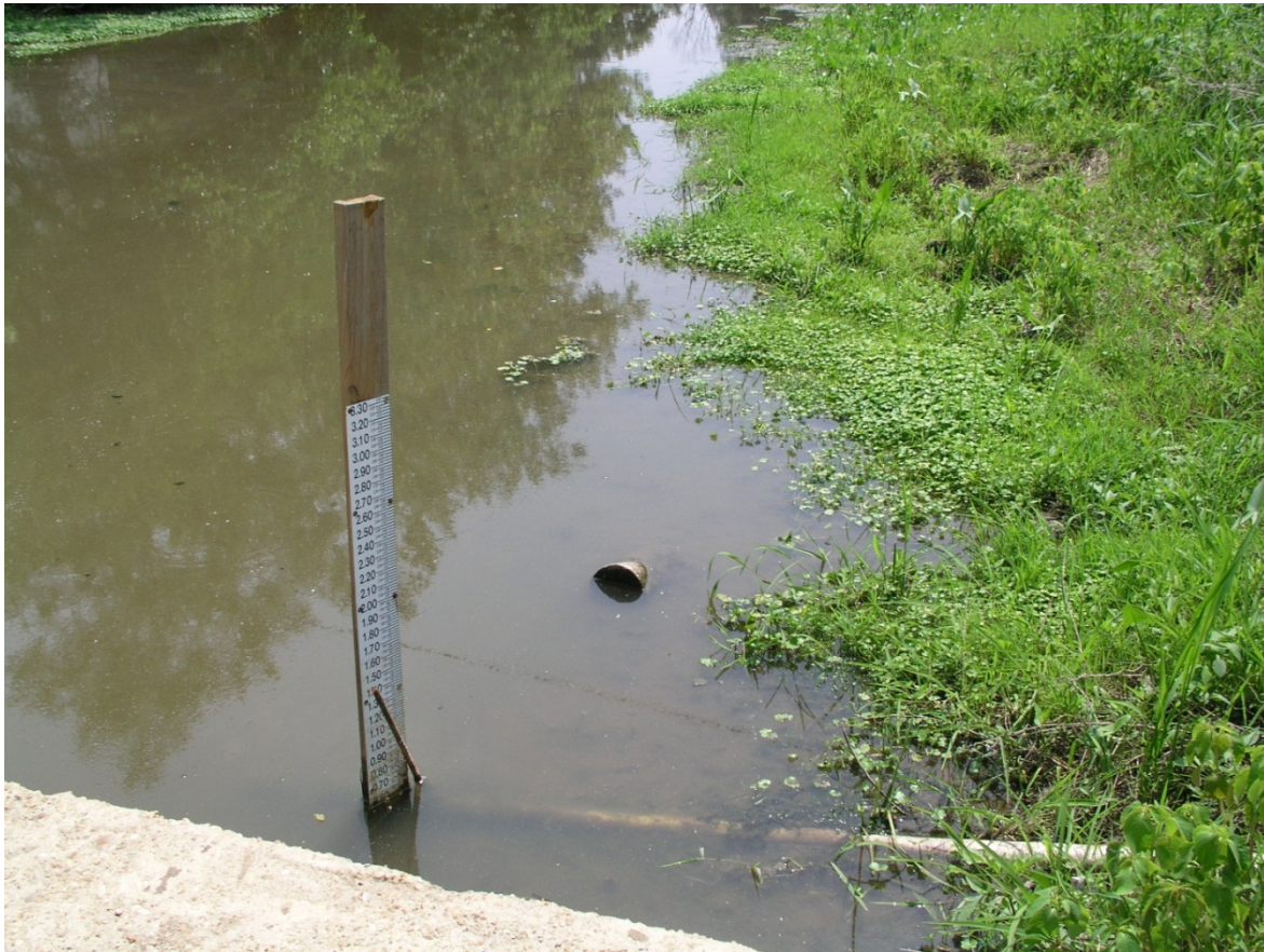
Figure 3-12. Staff gage in stream
