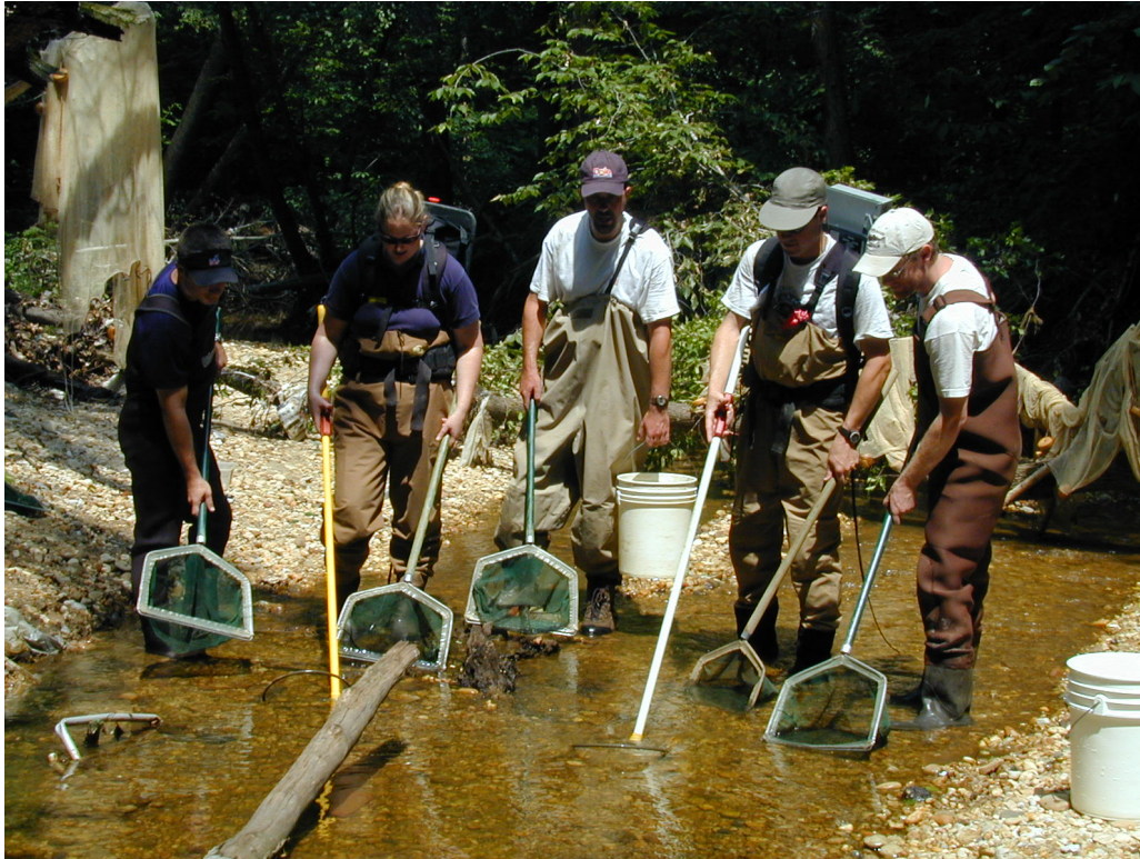
Figure 3-45. Backpack electrofishing (USEPA)
