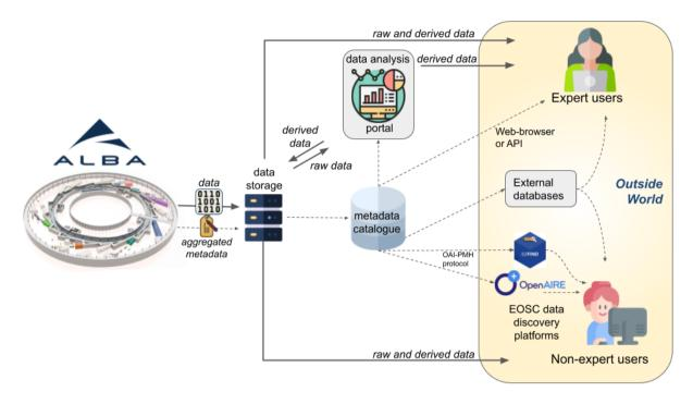
**Figure 3**: A high-level view of the (meta)data journey at PaN facilities. The flows of data and aggregated metadata are respectively shown using continuous and dotted lines.
