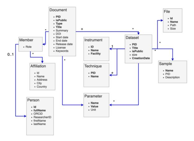
Figure 4: UML class diagram of the PaN search-API data model.
