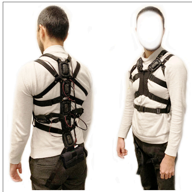
Figure 1. Image of the multimodal harness. There are nine actuators integrated on the structure: two on the clavicles, two on the ribs, and five along the spine. The straps are velcro-adjustable, two of which go around the legs to secure the last module against the body. The multichannel audio-haptics card is connected to the harness, situated below the last module on the spine.
