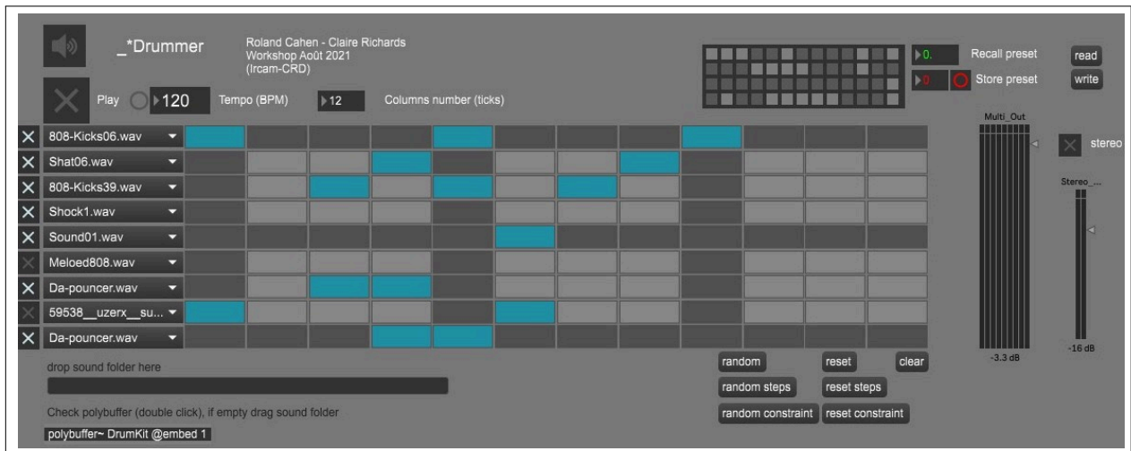
Figure 7. The Drummer interface seen in the Max environment. The sequencer tracks each correspond to one actuator position on the harness. Above the sequencer, there is a preset grid for saving specific drumming patterns.
