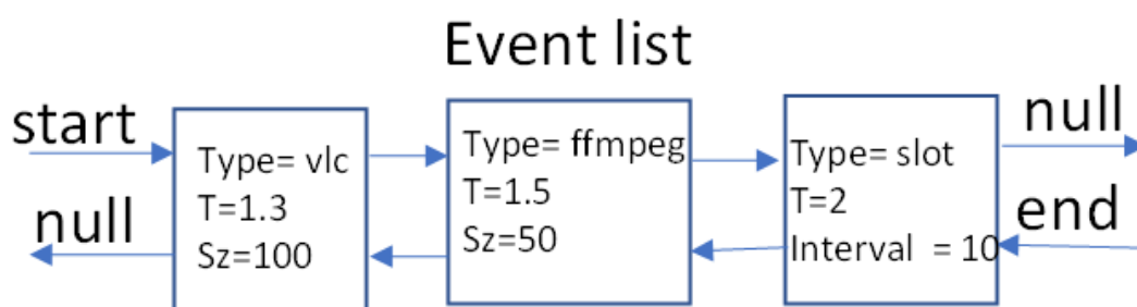
Figure 10. Event list to harmonise the times from different traffic traces and events occurring in network simulator
