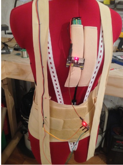
Experimenting with different placement positions for the Arduino boards and the battery
