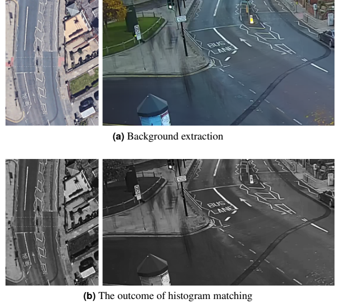
Figure 7. Histogram matching algorithm applied to the Leeds University Laidlaw Library (Parkinson Building) surveillance camera (right column), and the satellite image of the same location (left column).
