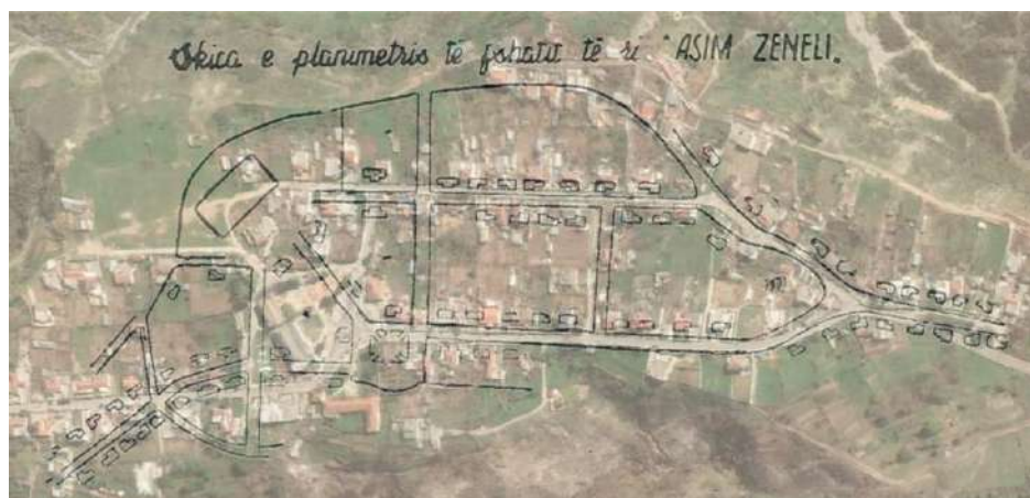
Fig. 6 Superimposition of the Google orthophoto (2021) with the handmade graphic sketch of the village masterplan published by Haxhiu in his 1963's article. Note the construction and permanence of the two parallel main roads and of many of the first houses built in the 1950s. F. Pompejano, 2021 (CC BY-NC-SA 4.0).
