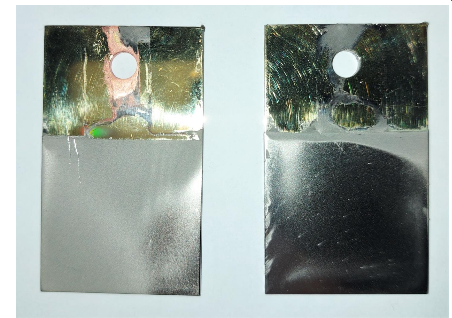
Figure 4. Comparison of images captured from coatings produced w and w/o the 3D printed barrier
