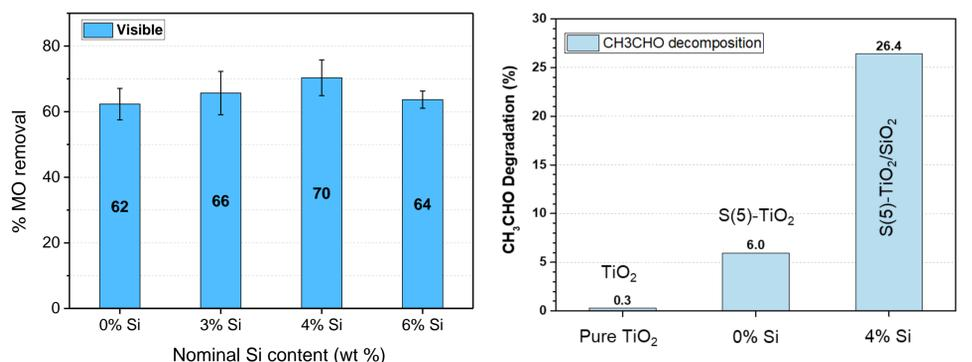
Figure 4. MO (t=5h) and aldehyde (t=1h) photocatalytic degradation under visible light.
