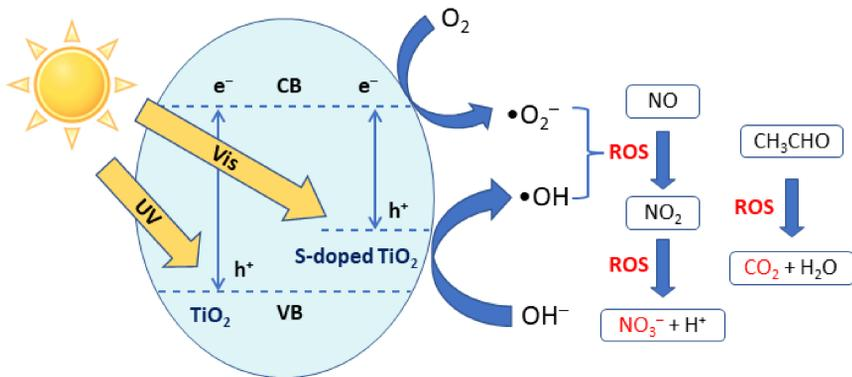
Scheme 1. ROS generation by TiO<sub>2</sub>-based NPs and photocatalytic degradation of pollutants.
