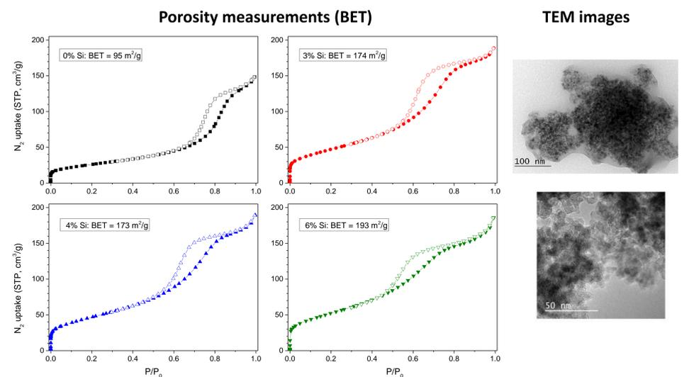
Figure 3. N<sub>2</sub> uptake for different SiO<sub>2</sub> content (left) and TEM images for 4 wt% Si (right).
