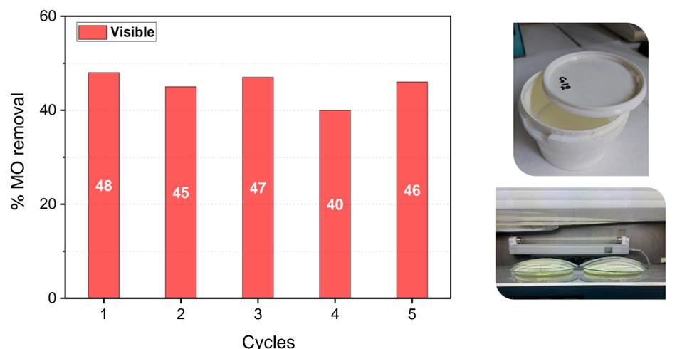
Figure 5. MO degradation under visible light over waterborne photocatalytic paint.
