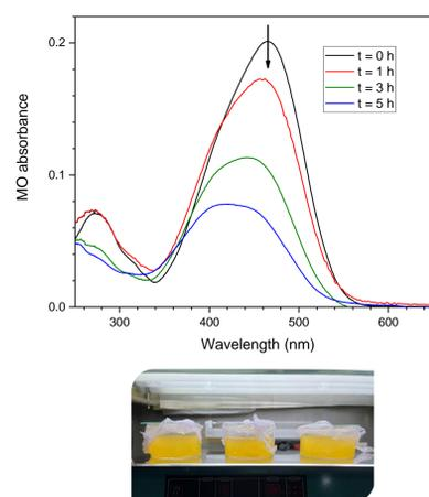
Figure 1. MO photocatalytic degradation in water under visible light, [MO]<sub>0</sub> = 2 ppm.
