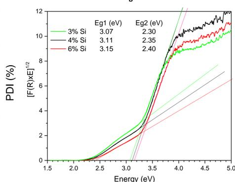
Figure 2. Hydrodynamic diameter (left) and Tauc plots (right) of S(5)-TiO<sub>2</sub>/SiO<sub>2</sub>-wt% Si NPs.
