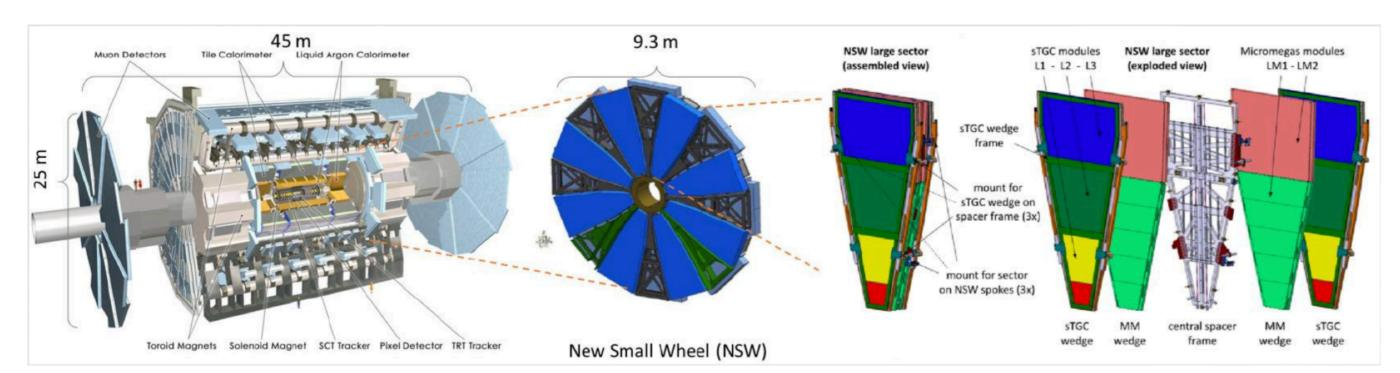
Tests are performed both during the detector construction phases and during the integration of modules into wedges, which are then combined together to make sectors.
