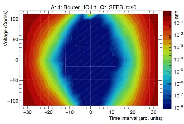
Detailed studies have been performed to mitigate the high noise by changing the grounding schemes, the improvements have been implemented and the noise levels have been greatly reduced.
