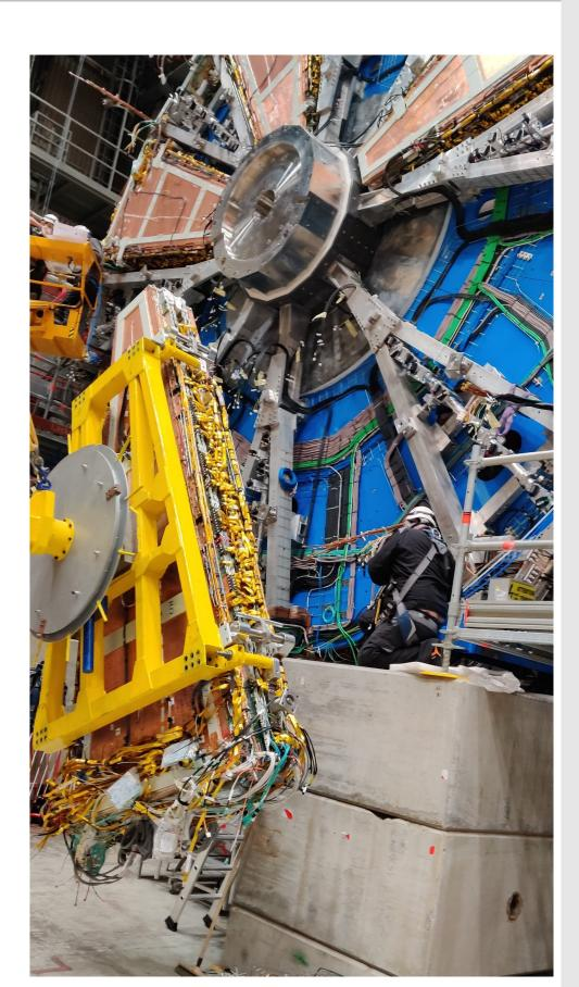
During the commissioning phase optical alignment tests of the chambers with respect to the alignment bars mounted on the support structure are performed in order to establish a grid in the ATLAS coordinate system.
