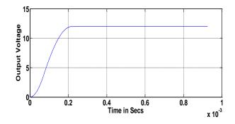
Figure 4. Output voltage of robust reaching law
