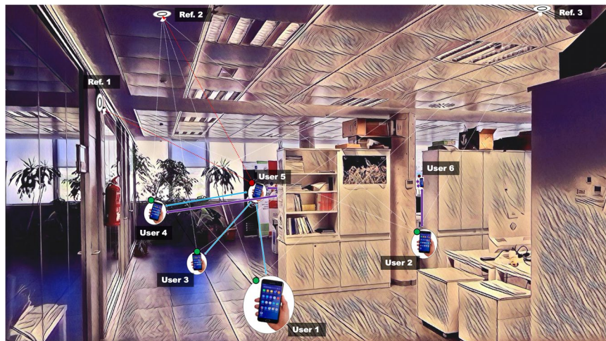
Fig. 1 Example of a Collaborative IPS scenario based on BLE and smartphones.
