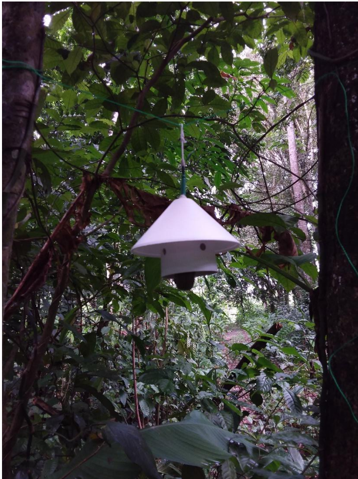
Figure 1: A temperature and humidity sensor within its radiation shield.
