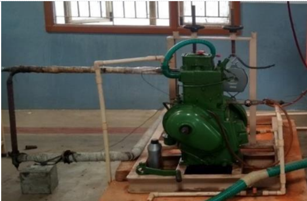
Fig 2: four stroke single cylinder diesel engine
