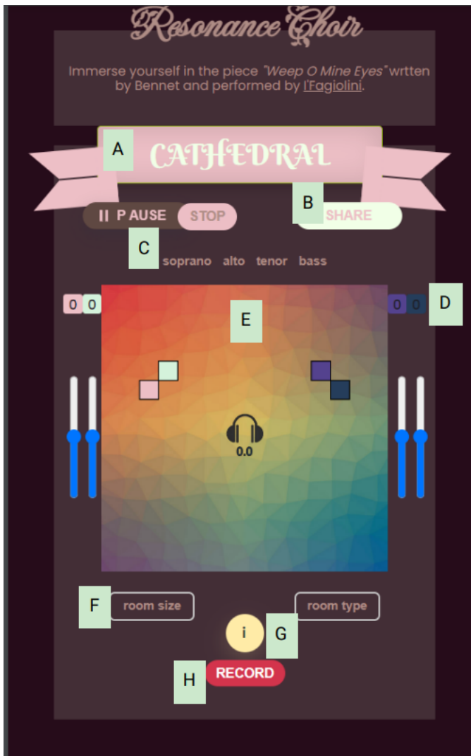
Figure 1: Screen shot of the Resonance Choir app with explanatory tags: (A) Listening location as chosen by the user; (B) Share button, which creates a URL comprising information about room property and recorded movements/muting of the singers; (C) Toggle buttons to mute/unmute the different singers; (D) Sliders to change the vertical position of the singers; (E) Interactive canvas where the four singers can be moved relative to a stationary listener (represented by the pair of headphones) by dragging the four rectangles; (F) Pop-over bubbles to change the room's preset properties (size of room and material of surfaces); (G) Information and how-to guide; (H) Record button which enables repeating and share the audio experience.
