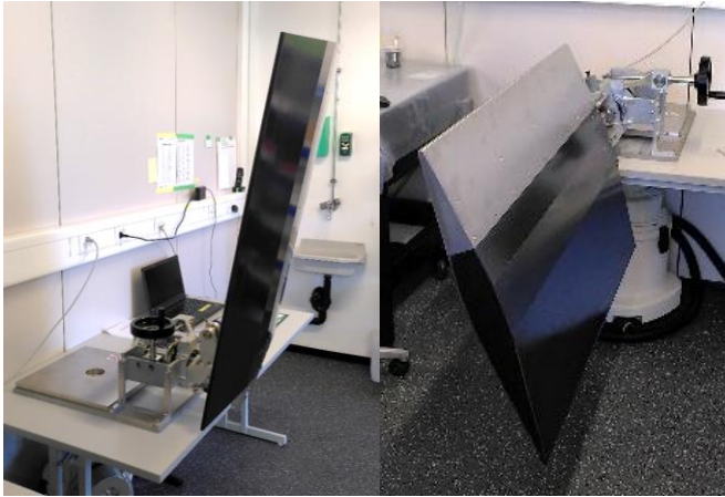
Figure 7: Control surface functional demonstrator test. Left: stowed configuration. Right: in operation in fully deployed configuration
