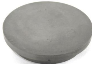
Figure 7: ZrB 2 -40vol.%HfB 2 -20vol.%SiC Ceramic side view (fixation pin hole visible)
