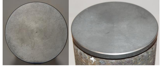
Figure 8: Ti 3 AlC 2 Ceramic top and side view (fixation pin and mounting shell visible)
