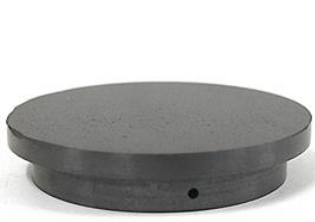
Figure 6: 3YSZ-10vol.%MWCNTs Ceramic side view (fixation pin hole visible)
