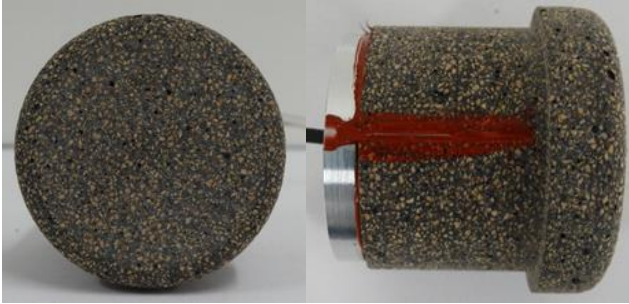
Figure 5: TPS05 cork sample, front and side view (instrumented, with sample holder plate mounted to the back surface)
