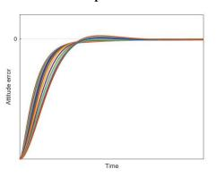
Figure 9 Pitch attitude controller time domain performance for different flight speeds; step response time history
