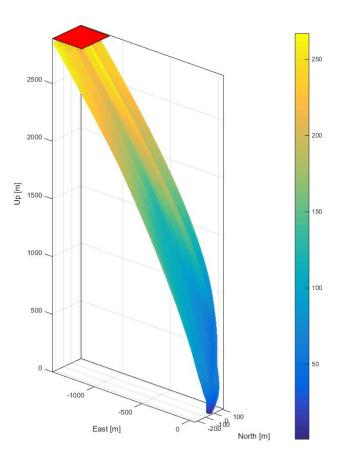
Figure 13 Trajectory path during the powered descent and landing phase
