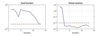
Figure 12 Convergence properties of the guidance solution, nominal case
