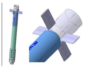
Figure 1 Baseline RETALT1 concept, with planar fins as main aerodynamic actuators [4]
