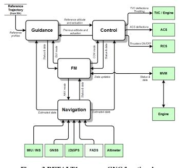
Figure 3 RETALT1 recovery GNC functional architecture
